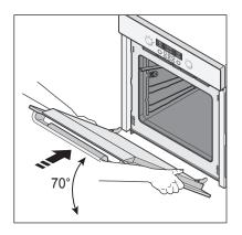
2. Rotate the door toward the horizontal line and flip the clips closed.
